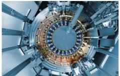
Gerresheimer uses state-of-the-art production facilities for the manufacture of primary packaging and drug delivery systems. Here, cartridges are formed from tubular glass. / More information via ots and www.presseportal.de/en/nr/9072 / The use of this image for editorial purposes is permitted and free of charge provided that all conditions of use are complied with. Publication must include image credits.
