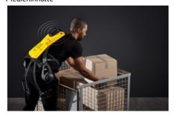
The 5th generation German Bionic Cray X exoskeleton provides up to 30 kg support per lifting movement for the lower back as well as active walking assistance for the legs. © German Bionic / Editorial use of this picture is free of charge. Please quote the source: "obs/German Bionic Systems"
