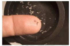
They seem to disappear into the grooves of a fingertip: The tiny pinions of a NOMOS watch caliber. Virtually all of the components for the in-house movements are manufactured at the NOMOS Glashütte production center. After all, even the best watchmakers can only build the best watches if they have high-precision parts.
