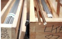
These rods will soon become watches: Three-meter long rods made of brass and stainless steel are delivered to NOMOS Glashütte. They will be turned, milled, and drilled on special lathes. The resultant tiny parts are then finished finely by hand.
