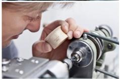
At NOMOS Glashütte, parts for movements are manufactured by machines that are precise down to a thousandth of a millimeter. Then each one is checked and finished by hand. Some are also lavishly decorated with traditional Glashütte sunburst finish—an elaborate process, one stage of which can be seen in the picture.
