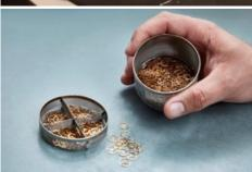
Fresh out of the CNC lathe machine at NOMOS Glashütte: Because the parts are so small, they are rinsed out of the machine in oil and left to fall into a sieve. Then they are cleaned and measured. It should be noted that without the people manning them, these machines would achieve nothing. It can take hours, oftentimes even an entire workday, to configure the machine for a new caliber part.
