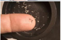
In the NOMOS Glashütte production center, the parts of the in-house watch movements are manufactured, including these tiny pinons for the various gear wheels of a caliber. In the watch world, working with the greatest precision is essential for every part. Even the best watchmakers can only build the best watches if they have high-precision parts
