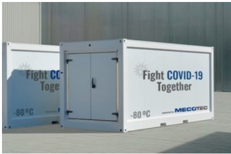
First Mobile Hybrid Container Solution made by MECOTEC with an active deep cooling technology for transport, storage and distribution of COVID-19-Vaccines down to - 80°C / -112 °F / Editorial use of this picture is free of charge. Please quote the source: "obs/MECOTEC GmbH"
