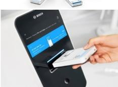
Running the test is easy: The sample is taken from patient?s nose or throat using a swab and placed without further preparation in the cartridge - which is then fully automatically processed in the Vivalytic analyser Editorial use of this picture is free of charge. Please quote the source: "obs/Bosch Healthcare Solutions GmbH"
