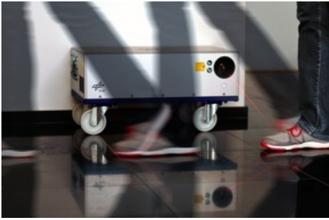
PHYLAX: Laser-based detection system for explosive detection. Source: DLR Editorial use of this picture is free of charge. Please quote the source: "obs/Lufthansa Consulting GmbH/DLR"
