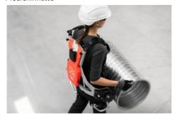
The German Bionic Cray X robotic exoskeleton is a human-machine system that combines human intelligence with machine power, by supporting and strengthening the wearer's movements, thereby reducing the risk of workplace accidents and load-bearing injuries. Editorial use of this picture is free of charge. Please quote the source: "obs/GBS German Bionic Systems GmbH"
