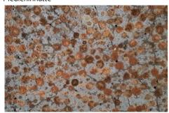
Concrete with desert sand pellets. Free use with photo credit MulitCON. Further text via ots and www.presseportal.de/nr/132903 / Editorial use of this picture is free of charge. Please quote the source: "obs/MultiCON GmbH"
