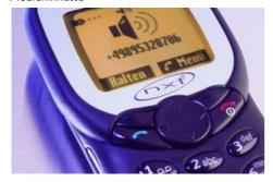
"Display Speaker Phone" the loudspeaker is integrated into the display of the phone. The integration will open-up more space for creative designs and technology.
