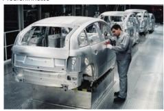
Aluminium expertise at Audi: Audi has now built more than 150,000 vehicles with aluminium body  $\theta$  including over 93,000 Audi A8 and just under 57,000 A2 models. Pictured: the Audi A2, the first volume-built car with Audi Space Frame (ASF).
