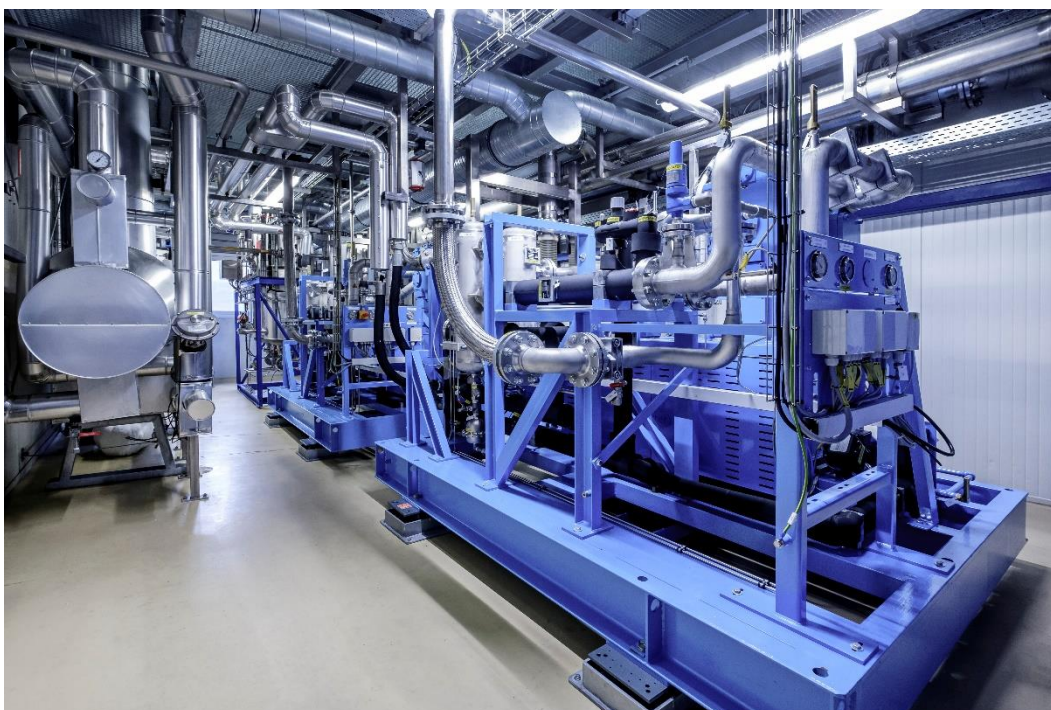
Image 2: The CO 2 recovery systems commonly used so far have a capacity of 100 to 8,000 kilograms of CO 2 per hour and are suitable for breweries producing between 200,000 and 16 million hectoliters of sales beer per year. Source: GEA
