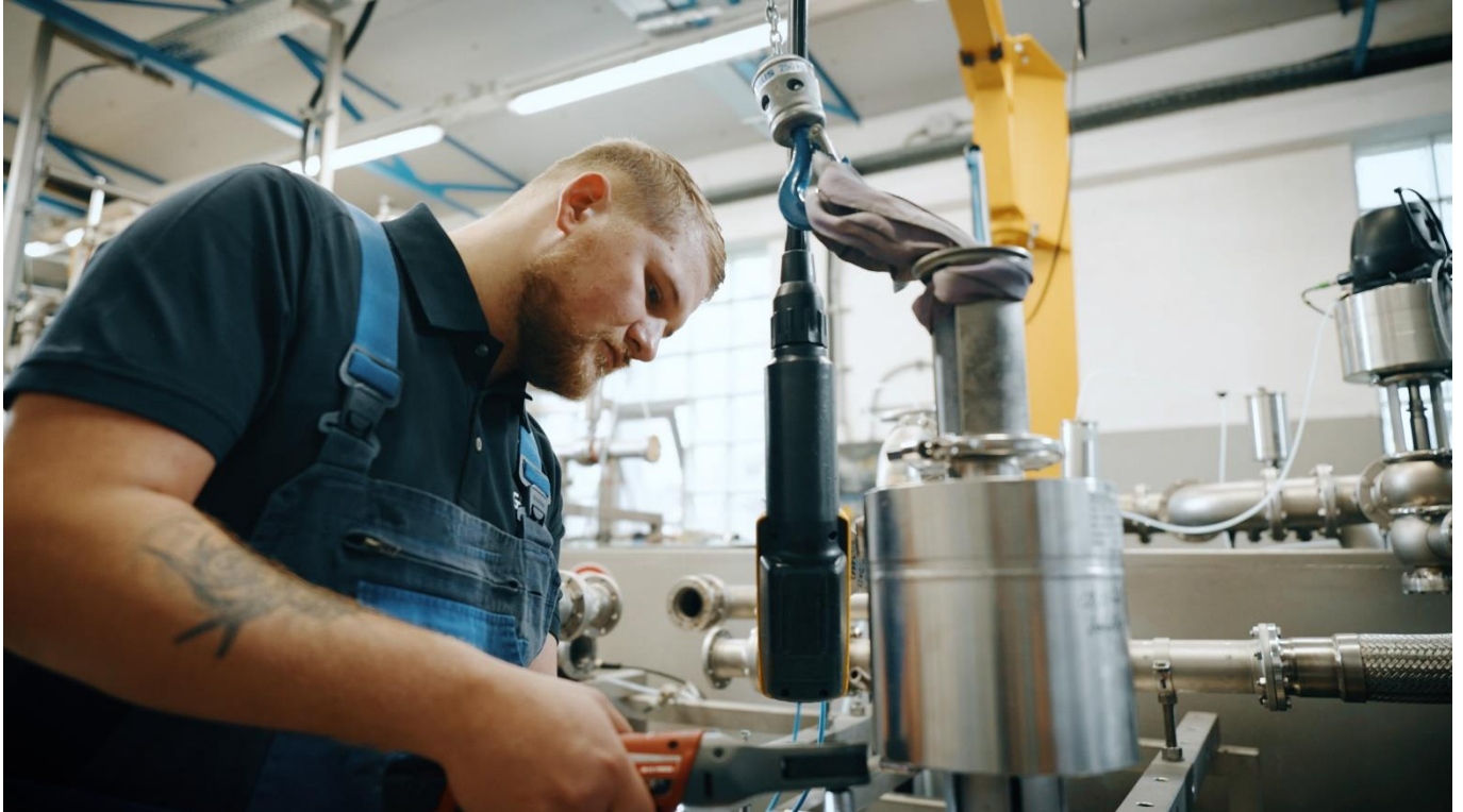
Fig. 1: Inadequately secured process plants are often the cause of accidents in production. This is why GEA now also equips the aseptic double-seat valves of the Aseptomag range with lockout-tagout (LoTo) devices. Source: GEA
