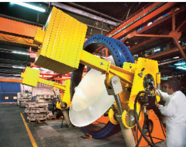
Carry some weight: new quarter-turn valve actuators help shut off large water pipelines.
