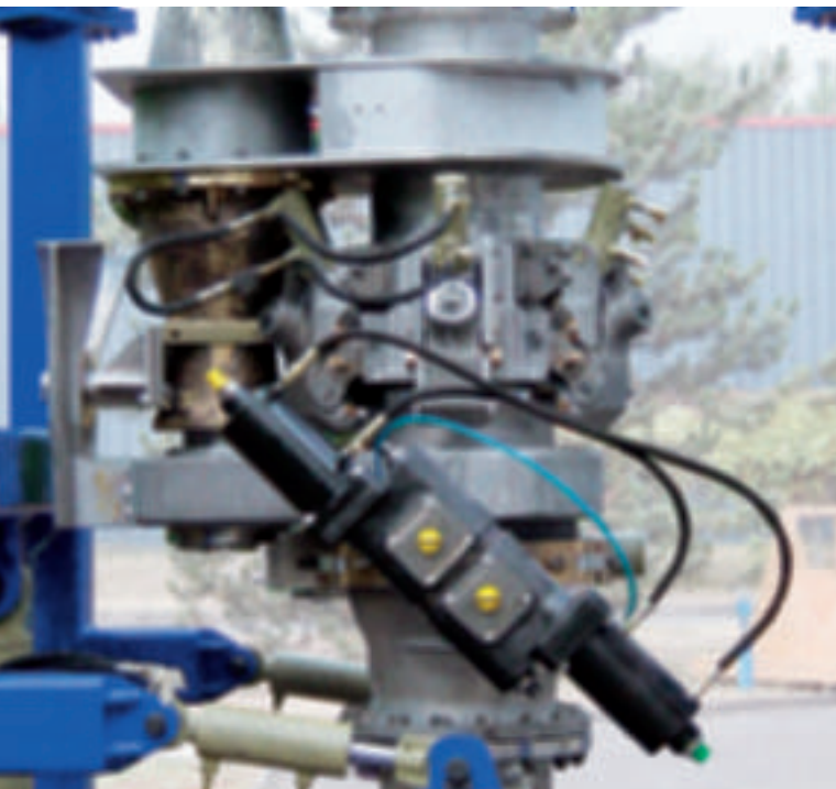
Ship to ship transfer: a KSB-developed coupling system is at the heart of the first flexible terminal for loading and unloading liquefied gas on the open sea.
