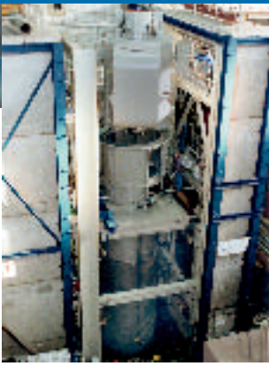
SEZ cooling water pump on the test rig.
