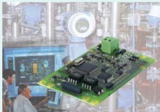
Fieldbus integration kit: Compact FF interface for HART devices
