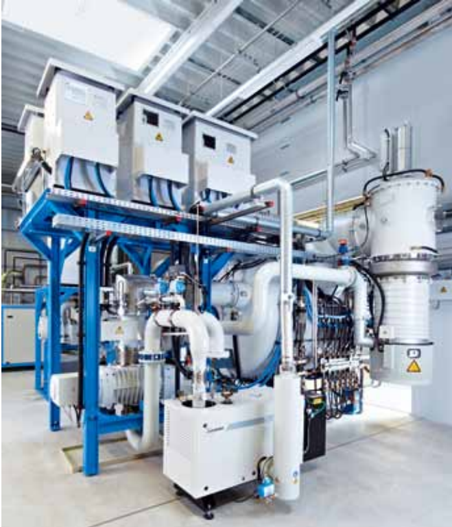
Top: The new brazing furnace's CFC heating elements Left: View of the back of the brazing furnace with its high vacuum pumping station
