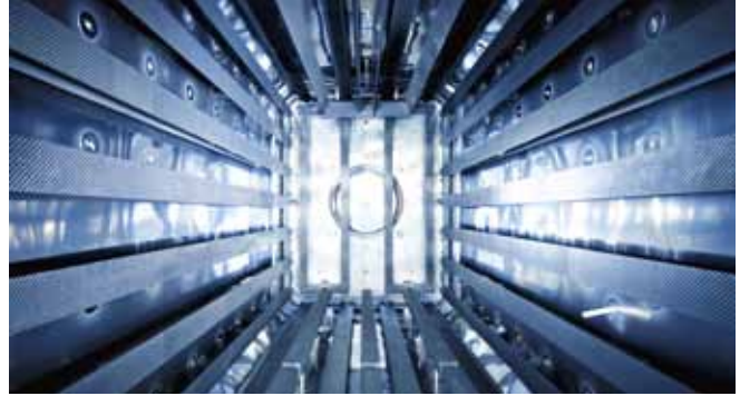
Top: The new brazing furnace's CFC heating elements Left: View of the back of the brazing furnace with its high vacuum pumping station
