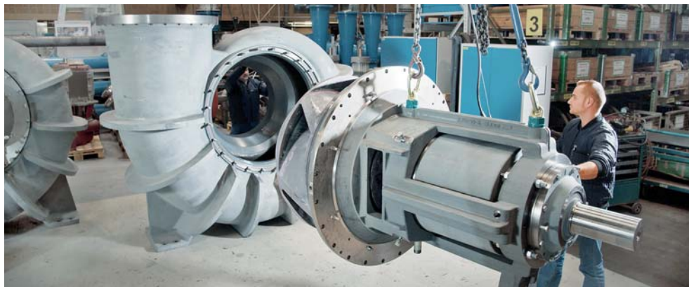
The first pumps to feature extremely hard-wearing polymer impellers were produced for a flue gas desulphurisation system in South Africa.
