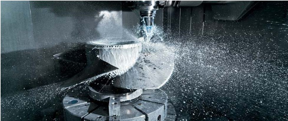
KSB pumps with propellers (shown here during processing) are used around the globe for flood control and transporting waste water.
