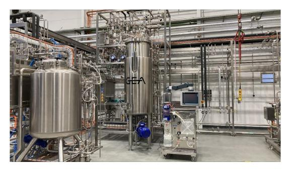
For the first time, the new food experts will discuss their perfusion platform – a key technology for state-of-the-art upstream bioprocesses that also enables continuous processing in cell cultivation and precision fermentation. This solution consists of GEA Axenic bioreactors and the GEA kytero single-use separator. Source: GEA
