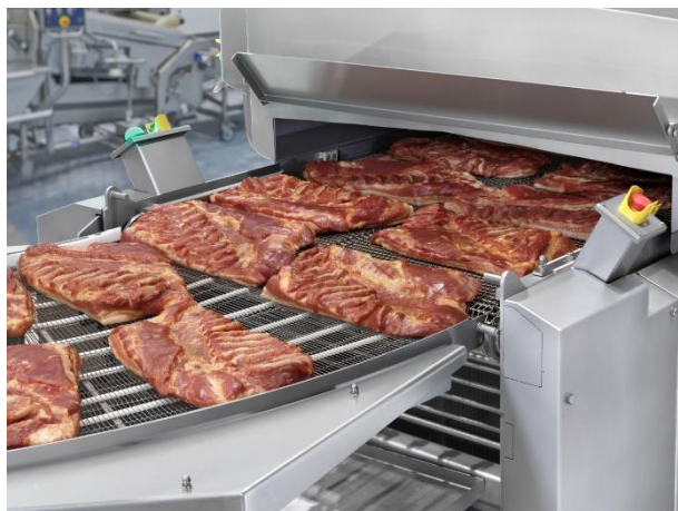
Pic. 2: GEA CookStar 1000 GEN 3 outfeed with smoked bacon bellies (GEA)
