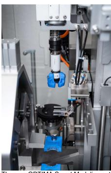
The new OPTIMA Smart Moduline sets new standards in the mid-range performance segment for cosmetics applications and will be on display for the first time at Interpack. This shows a closing module that can be flexibly equipped with format parts from a 3D printer. (Source: Optima)
