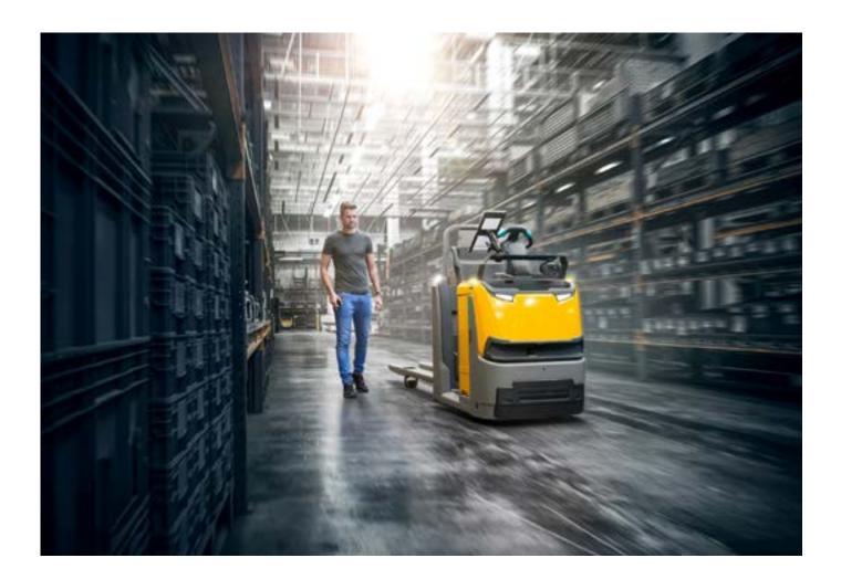
They are ideal for transporting bulky, heavier items and can easily be combined with new interaction devices like Voice Picking. Their sheer size allows operators to stack boxes and the follow-me mode saves time as operators don't need to step on, drive and step off the vehicle anymore between goods picked. This technology increases the picking rate and reduces occupational hazards.
