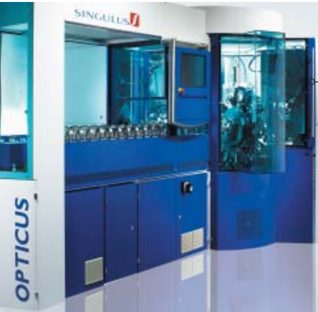
OPTICUS: The technology for inline optical coating of eyeglass lenses will be presented at MIDO/Milan in early May
