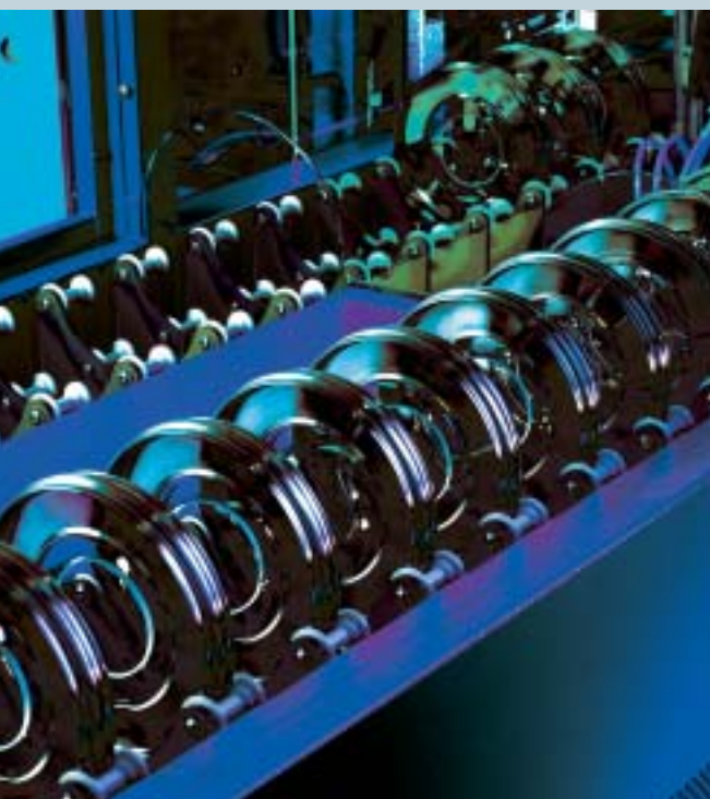
OPTICUS: The technology for inline optical coating of eyeglass lenses will be presented at MIDO/Milan in early May
