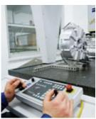
Contours, surfaces, roughness and roundness are quality features that are precision-checked in our products. Before shipment, all the engines are tested as a complete system on the dynamometer to remove any faults and assure the quality of manufacture.
