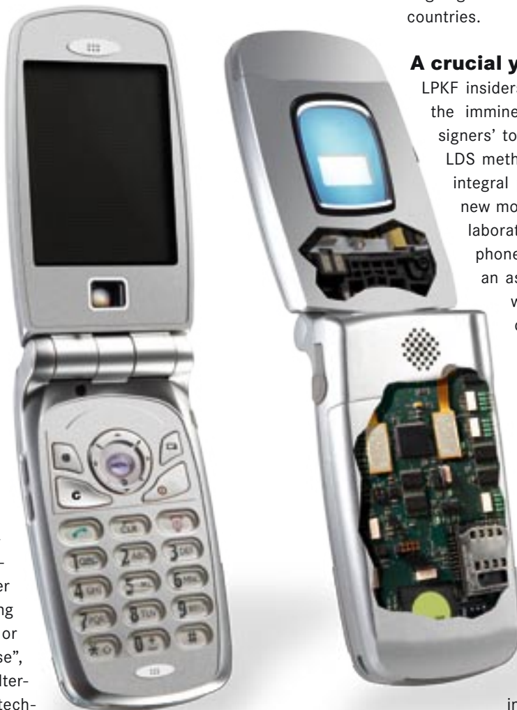
Mobile telephone with 3D-MID antenna
