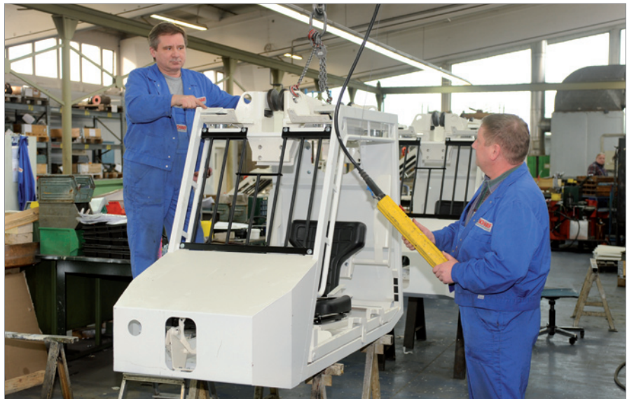
Specially trained experts assemble a monorail hanging railway in Hamm
