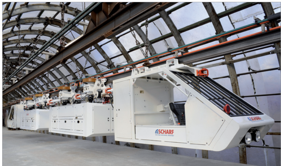
EMTS, the electric monorail hanging railway offers an alternative to diesel engines
