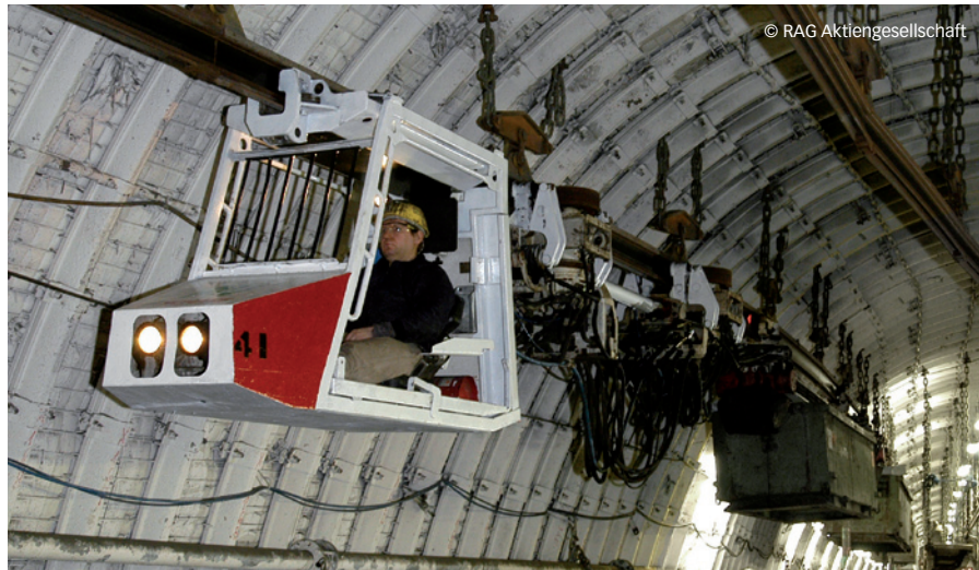
Monorail hanging railway at work carrying a load
