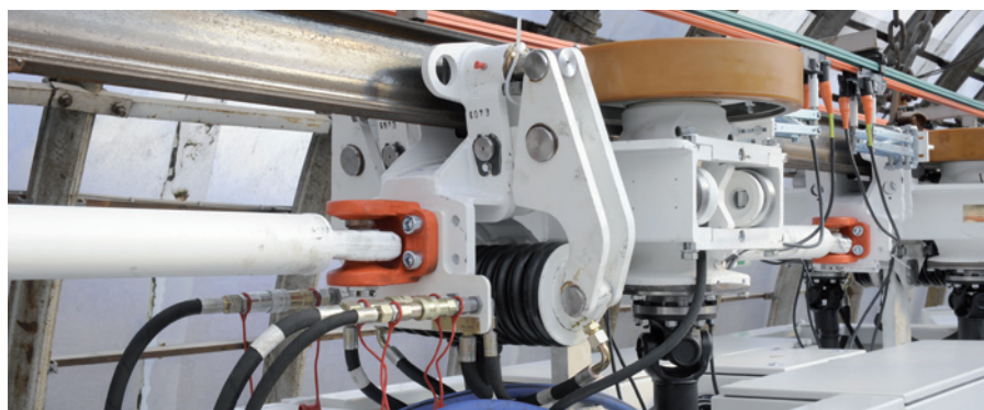
Friction wheels are the mostly used means of power transmission
