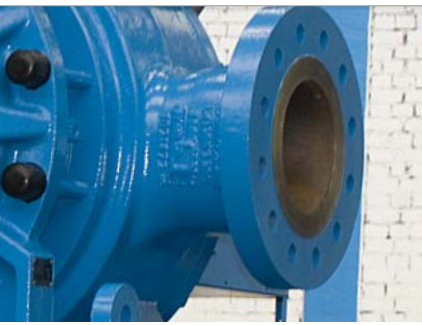
High-pressure pumps for a seawater desalination plant in Australia
