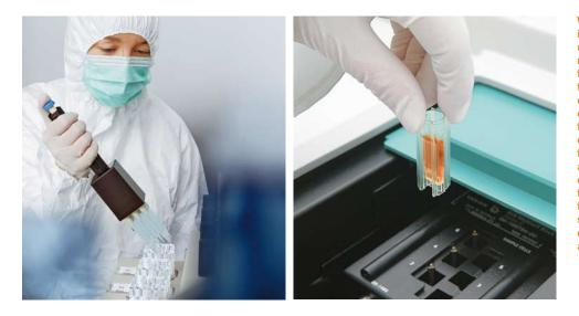
Wacker Biotech GmbH in Jena, Germany, uses genetically optimized E.coli bacteria to produce active proteins for pharmaceuticals. The final analytical step includes testing whether the desired protein contains the right amino acids in the right order. whether it has folded into the right three-dimensional shape and whether it displays the desired activity.
