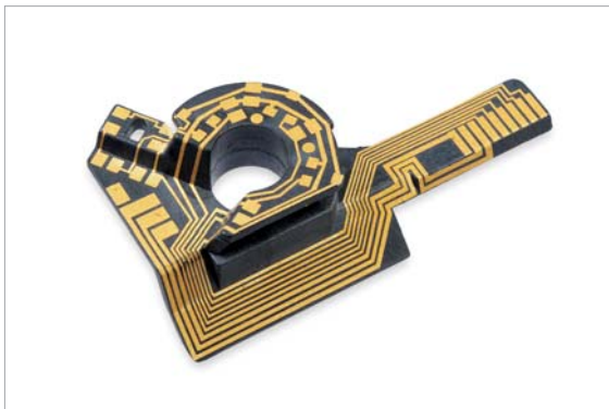
Circuits directly on plastic components: innovative components through laser direct structuring (LDS).
