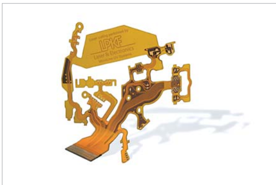
Intricate and precise: the PCB production laser cuts complex contours cleanly with no burrs.
