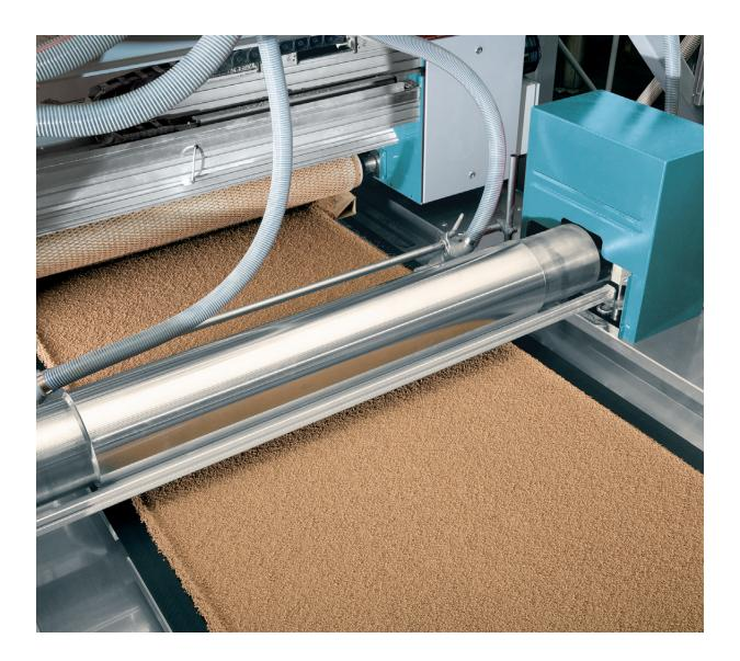
Thin layers: a double-belt press compacts the cork and VINNEX® binder pellets at about 180 degrees Celsius to form an endless cork-plastic sheet. In the height of summer, stone flooring feels refreshingly cool to hot feet – in chilly months, though, the prospect of treading on cold tiles is less enticing. Only bathrooms and kitchens boast easycare stone flooring. Living rooms and bedrooms have it "cozier," with carpeting or wood creating a warmer sensation.
