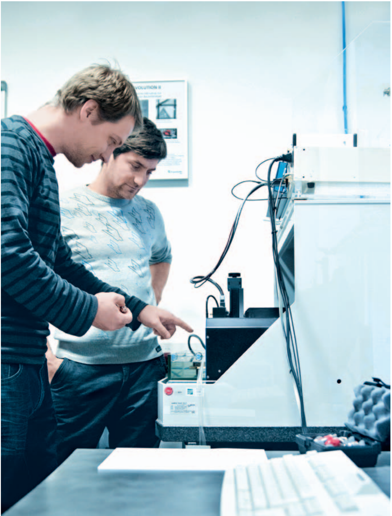
The SAM laboratory at the Fraunhofer Institute: Besides being equipped with a SAM EVOLUTION from PVA TePla Analytical Systems, the institute also has a high-resolution SAM microscope that is effective at up to 2,000 MHz and a prototype of the new modular SAM 2000, combined with an optical reflected light microscope and an inverted microscope.
