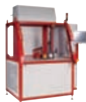
Helium leak detection systems
