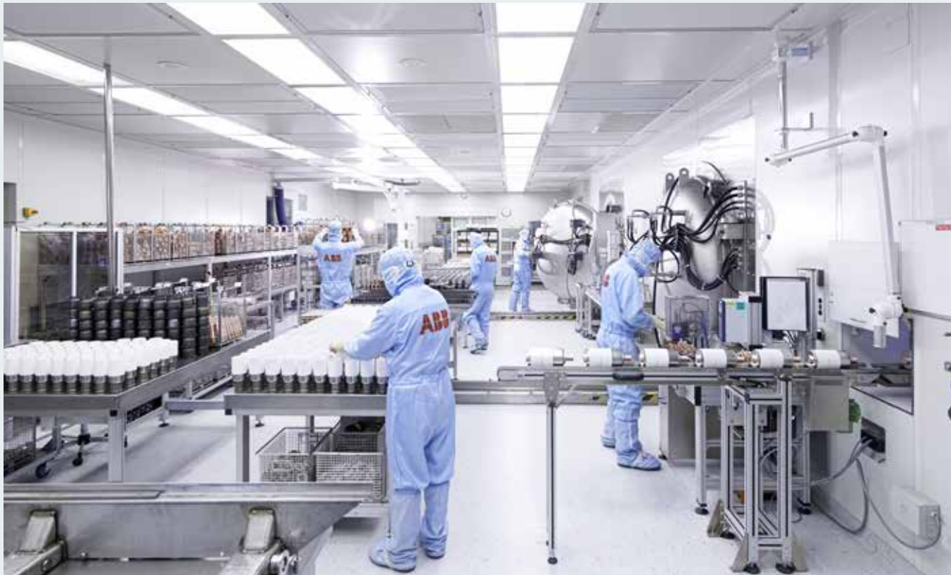
Vacuum Interrupters are Prepared for the Brazing Process
