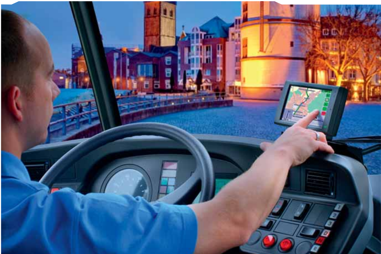
Drivers' benefit: on-board computers with touch screen facilitate work – from radio communication to driver navigation.
