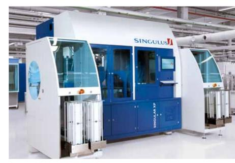
02 SINGULAR XP vacuum deposition machine for the coating of the rear side of crystalline solar cells
